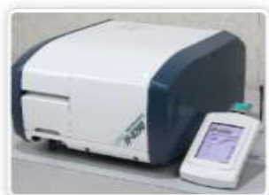
Spectrofluorometer FP8200, Jasco, Japan
